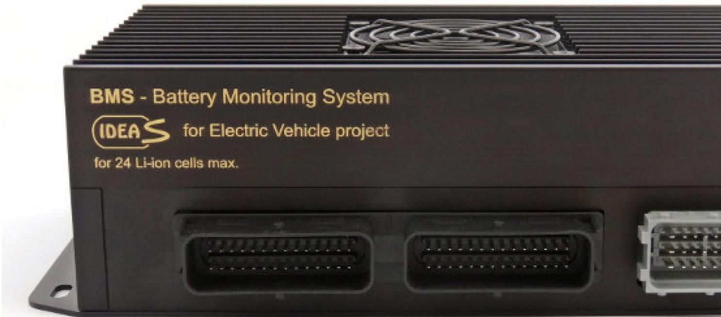
Front view of new prototype Battery Monitoring System device.
