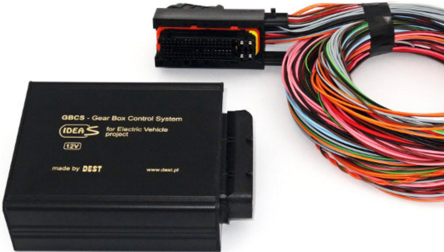
Prototype Gear Box Control System
